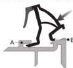
Fig 1 Insert back leading leg into the bead retention slot
