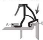
Fig 2 Push downwards or tap with rubber mallet
